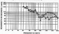
FIGURE 4 — Directivity vs Frequency
